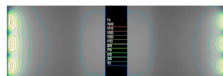
Figure 3-16 Bilateral Plan Rendering with Illuminance ISO Contours
