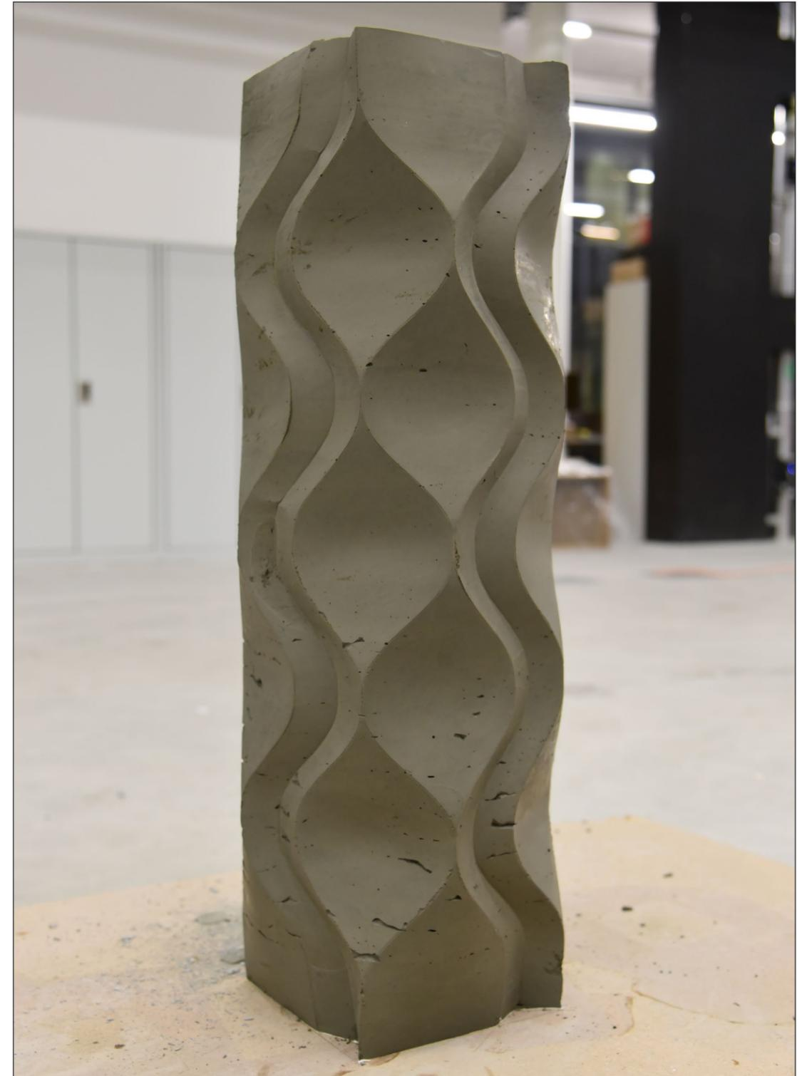
Ultra-thin folded paper formwork (0.5 mm thickness) with set on demand concrete casting (2019 - Present)
