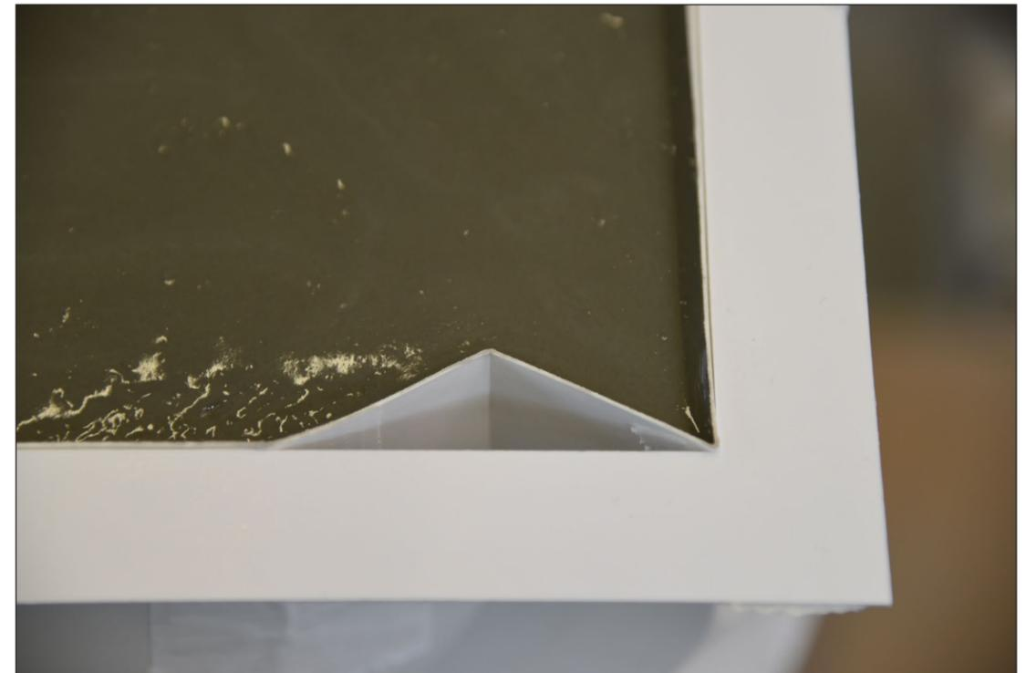
Ultra-thin folded paper formwork (0.5 mm thickness) with set on demand concrete casting (2019 - Present)
