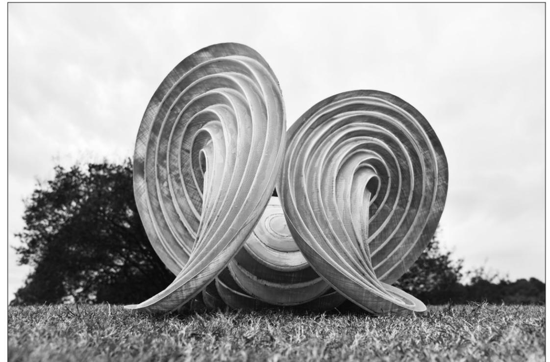
Folding fiberglass along curved creases. The 8ft in diameter saddle is composed of twenty concentric circles. Principal Investigator: Joseph Choma, Clemson University (2018)
